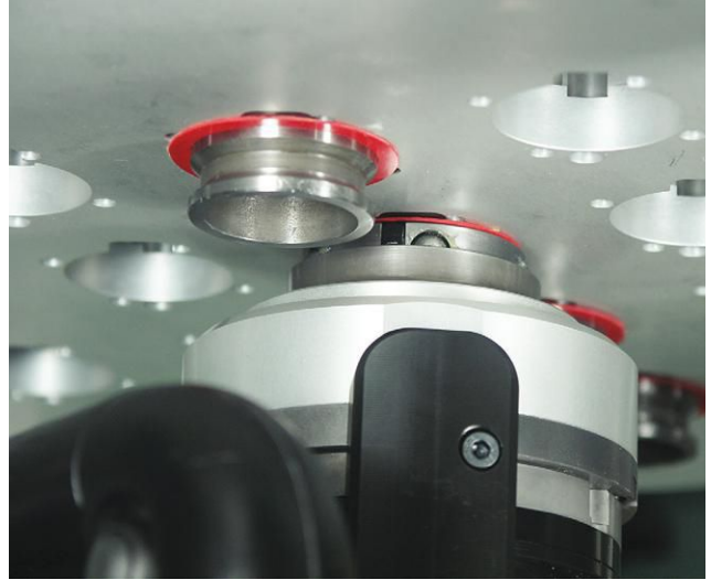
A portable Novator orbital drilling machine and a close-up view of the drill jig and bushings to which the machine is clamped for each hole. RFID tags in the drill plate and machine ensure only the correct hole is drilled (Provided by Novator)
